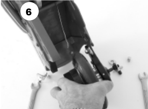
6. Pull the old wheel out. Note the arrangement of the hardware sequence below (7 ~ 10)
