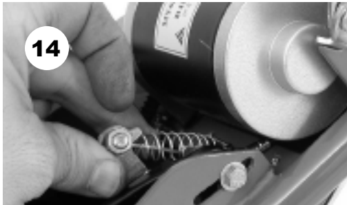
14. Insert the brake spring and thread the cable wire into the cable anchor. Thread the cable to its original position and tighten securely.
