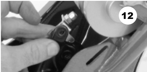
12 & 13. To hook up the brake anchor arm and cable. Align the cable guide adjuster and install the spacer and bolt. Do not tighten until after step 19.
