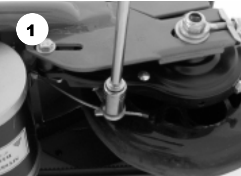
1. Loosen brake cable anchor and remove.
