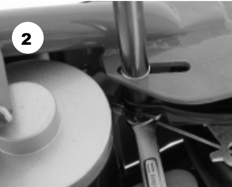
2. Loosen brake arm anchor and remove
