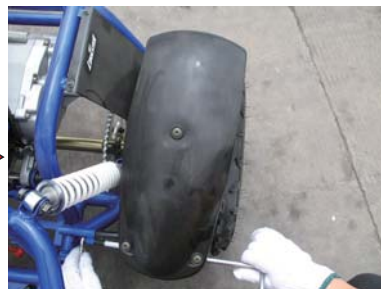
8、Install rear fander
