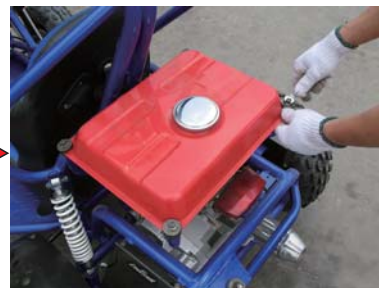
17、Intall fuel tank
