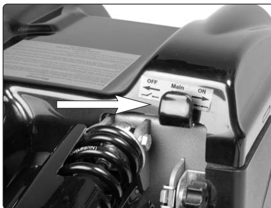
Main fuse in the ON position
