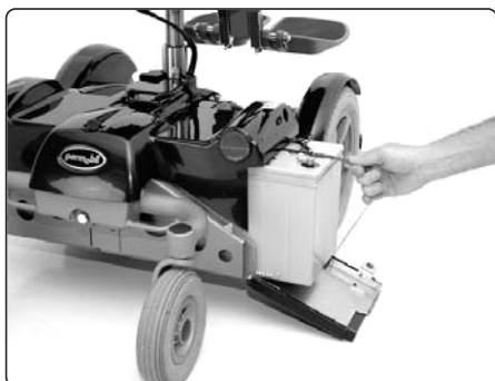
Disconnect the battery's first connection
