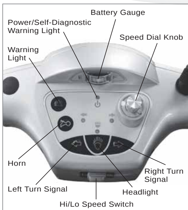
Figure 2 - HS-890 Control Panel
